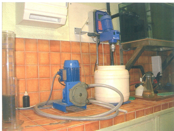
PMA Series used for sampling in the control process at a waste water treatment plant
